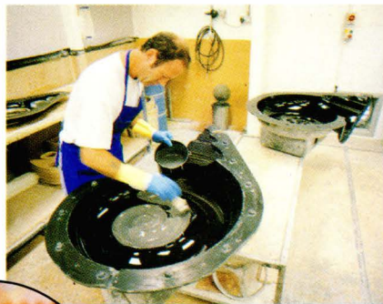
Above: the 300mm metal-coned bass driver is fixed in a gel damped tube. Right: layering up the GRP moulds. Below centre: an early prototype model with flat sides and the so-called pixie cap. Bottom: fully adjustable cross-over.
