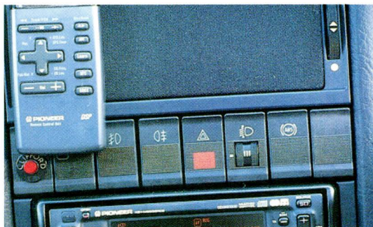
The hand-held remote control (top) makes switching between the various DSP modes on the move far easier.
