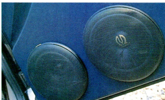
A three-way, full-range component speaker set driven by a GM-1200 amplifier finds a home in the front doors.
