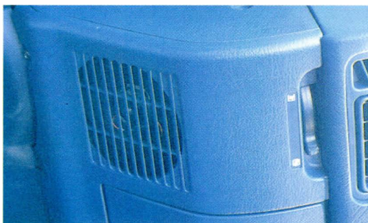
Component speakers in the front of the car are hidden from prying eyes behind the standard trim panels.
