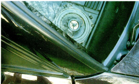
Front speakers fire up into the car windscreen; a centre channel driver (not shown) is in the middle of the dash.
