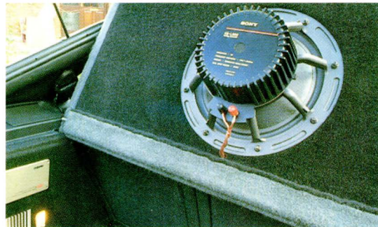
That's one big subwoofer, a 12in XS-L300 in fact, and it is very neatly installed in a custom-built rear parcel shelf.
