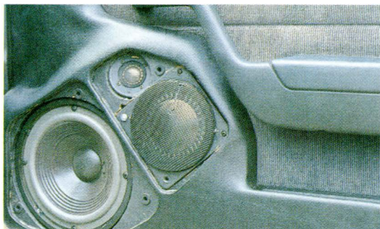
Front doors are bursting with drive units, including an 8in subwoofer, each set driven by a 400 watt amplifier.
