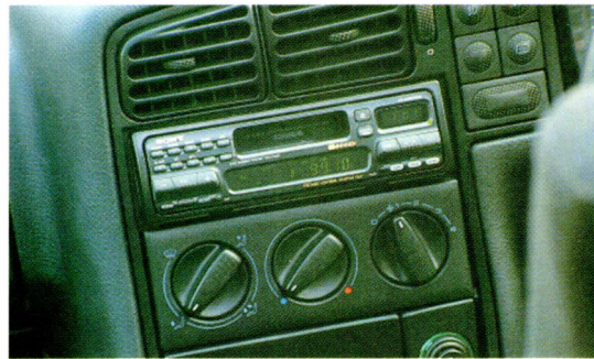
The Sony XR-U800 plays tapes, has an RDS EON tuner, and controls both the CD changer and digital processor.
