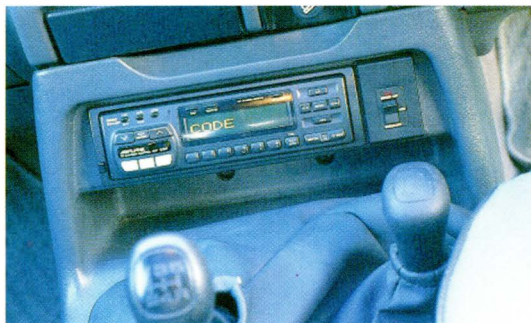
The sleek and unobtrusive 1310R acts as a controller for the CD changer and boasts an RDS EON radio tuner.
