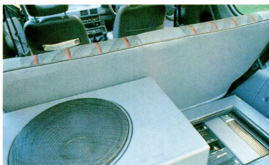
Creating the perfect image is the job of the 3681 digital crossover with time alignment, right of the subwoofer.
