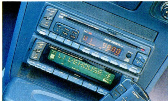
The CDC6700R (top) plays single discs and controls the CD autochanger; effects are via the DSP959E (bottom).
