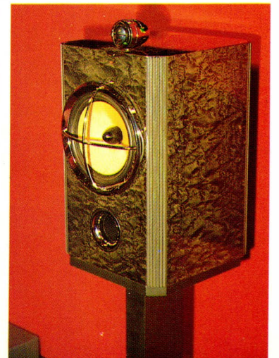
Below left; one of several colour options in Sony's German ES range, and right, B&W's Silver Signature has all silver wiring and coils, and comes complete with external crossovers and silver speaker cable.
