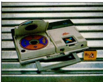
The PC-Engine CD-ROM system in its carrying case/interface unit - CD player on left, games console unit on right
