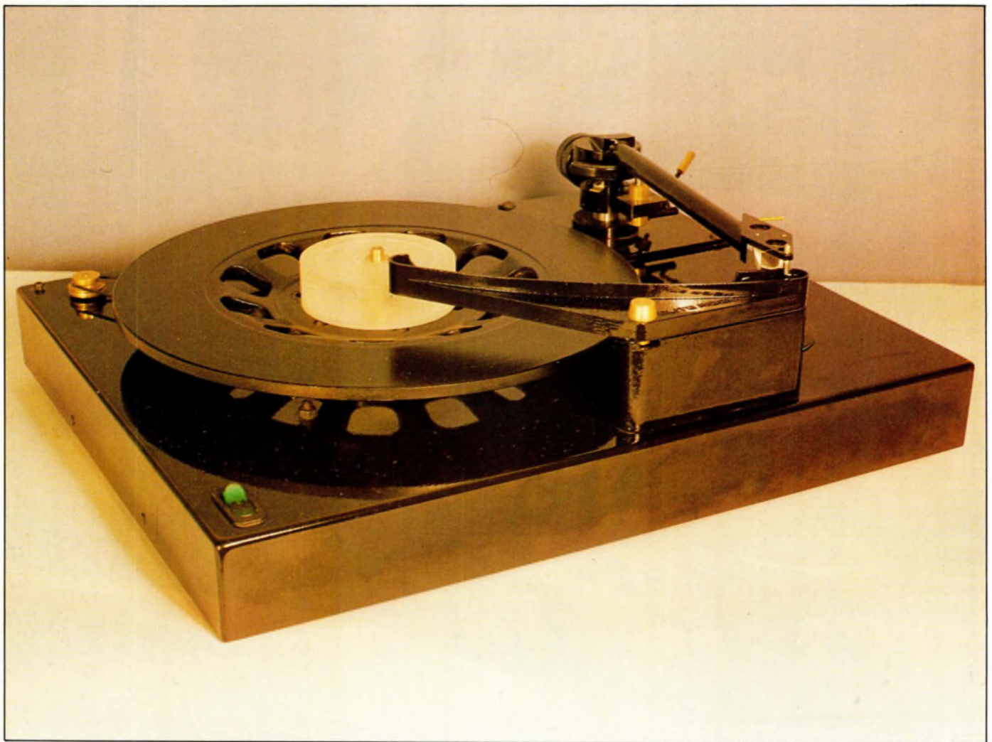
The 'Meitnerised Rock', incorporating disc brake courtesy of Yamaha motorcycles.
