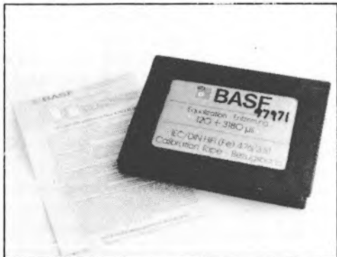
Figure 1. BASF calibration tape, used to check adherence of replay response to the current IEC standard
