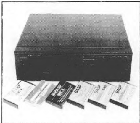
Figure 4. IEC Primary Reference tapes, shown here with the Nakamichi ZX-9 used as a 'reference' cassette deck in this book. Chosen by international agreement, these tapes have electrical characteristics which other tape manufacturers have accepted as a standard. The Primary References are BASF ferric, BASF Chrom II chrome, and TDK Metal, and have been used for all deck frequency response measurements in this book
