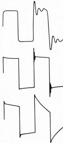
10kHz squarewave left: 8Ω load right: 8Ω + 2µf load
