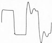
10kHz squarewave left: 8Ω load right: 8Ω + 2μf load
