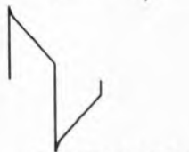
100Hz squarewave left: 8Ω load right (if appropriate): 8Ω, LF filter 'in'.
