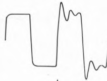
10kHz squarewave left: 8Ω load right: 8Ω + 2μf load
