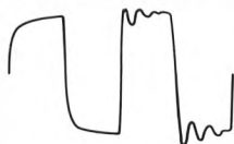
10kHz squarewave left: 8Ω load right: 8Ω + 2µf load
