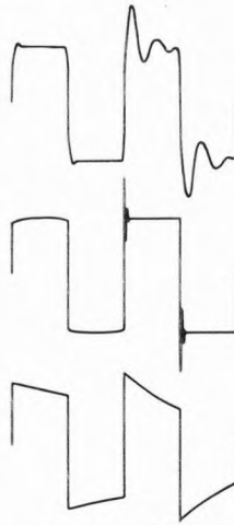
10kHz squarewave left: 8Ω load right: 8Ω + 2μf load
