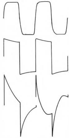
10kHz squarewave left: 8Ω load right: 8Ω + 2μf load
