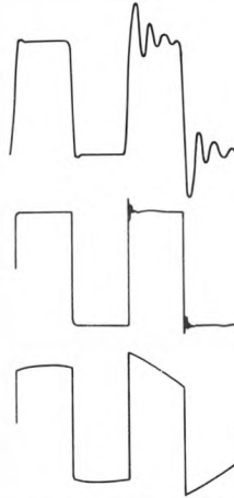
10kHz squarewave left: 8Ω load right: 8Ω + 2μf load
