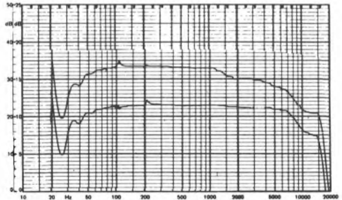
Sony TC209SD: Sony FeCrO2 Dolby In Sony TC209SD: Sony HF Dolby In
