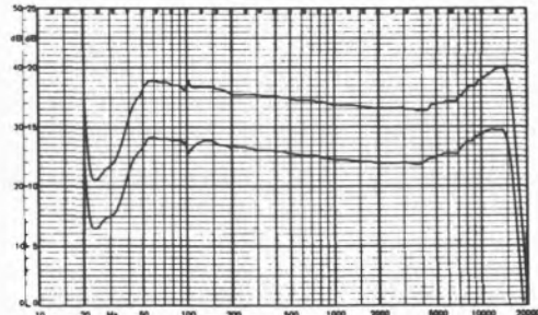
NEAL 103: TDK Kr Dolby In (after tweak bias reduction) NEAL 103: TDK Kr Dolby In (before tweak bias reduction)
