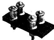
Fig. 20. Ebonite former and side supports for the transformer shown in Fig. 18. At the right is the top plate with the four terminals
