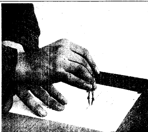
Fig. 6. With the aid of dividers the degrees are marked off at intervals round the crescent
