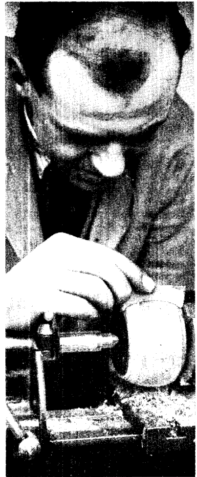
Fig. 8. Accuracy must be tested from time to time during the turning operation. In this photograph a template is being applied for this purpose
