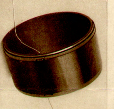
Fig. 12. No. 24 gauge wire is wound on ebonite for the inductance
