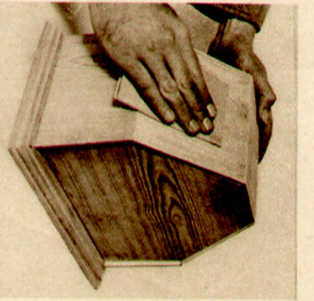
Fig. 11. Sand-papering the cabinet before staining and polishing
