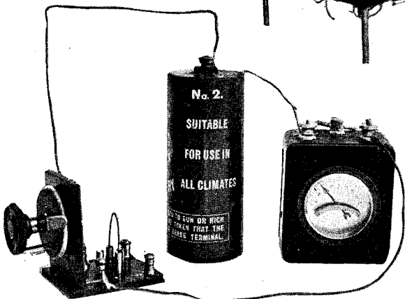
Fig. 6. Placed in series with a battery and valve unit is a galvanometer, which is used to test the continuity of the filament circuit
