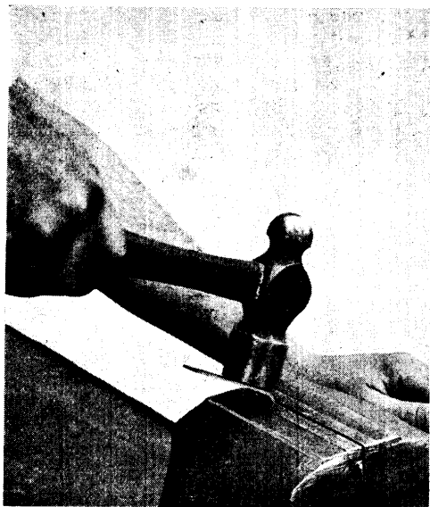
Fig. 1 (left). Brass strip is bent with a hammer, holding the work in a vice. The blows should be delivered gently a small distance from the bend. Fig. 2 (right). Laminations can be riveted together to form a switch arm. The operator is seen flattening the small copper rivet with the round side of the hammer
