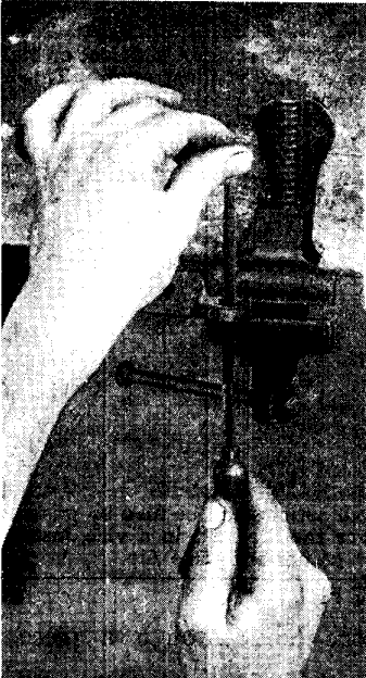
Fig. 4. When casing out a hole with a round file the worker's hands appear as shown here
