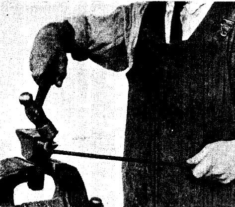
Fig. 7. First stage of forming a hook. The heated end of the rod is being hammered round the beak of the anvil
