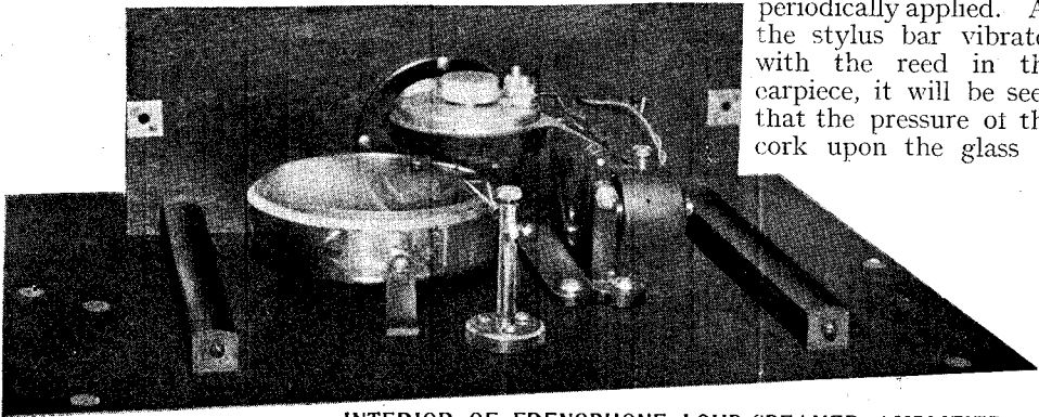
INTERIOR OF FRENOPHONE LOUD-SPEAKER AMPLIFIER
