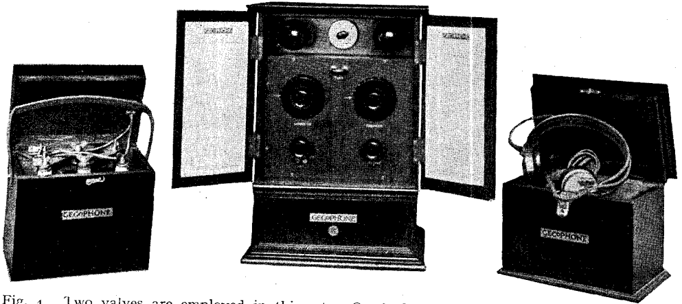
Fig. 4. Two valves are employed in this set. On the left is the low-tension battery and on the right the high-tension battery, together with a compartment for the telephones
