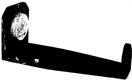
Fig. 8. One way to support the tube for a loose coupler is here shown. Note the circular cheek
