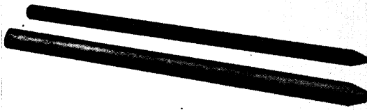
Fig. 1. Arc lamp carbons. They are made from lamp-black, prepared from creosote oil, and afterwards consolidated with tar and other materials, and baked in crucibles
