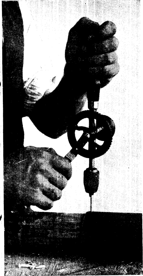
Fig. 3. Holes should be bored in a cardboard tube in this manner for the ends of an inductance coil to pass through
