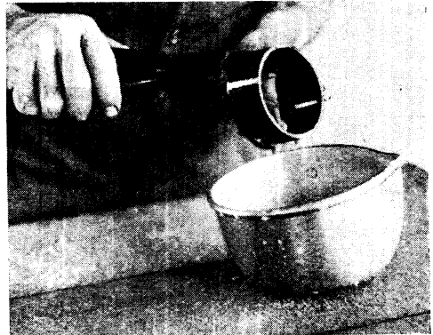
Fig. 5. Molten paraffin wax is prepared, and the former, held by pliers, as in the illustration, is dipped in the bath
