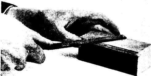
Fig. 11. Angle strips are finished off by filing the edges true and even
