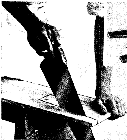
Fig. 33. Side pieces are cut out first and the legs made by sawing out a blunt V-shaped piece of the material. Fig. 36 (top, right). Legs for the cabinet may here be seen more clearly. A complete side is shown with the outside uppermost. Fig. 37. Grooves are sawn for the shelves, as illustrated. One groove is completed, one is sawn but not chiselled out, and one is being sawn
