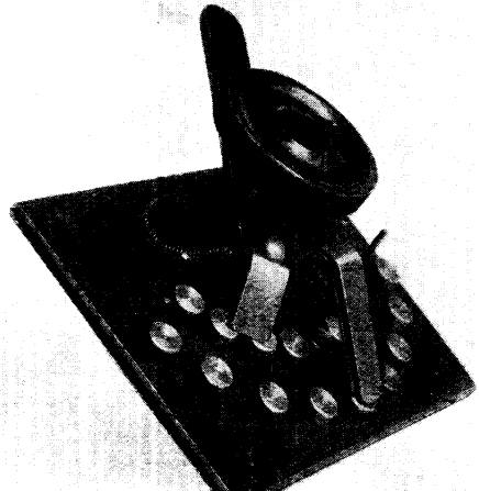
Fig. 2. Multi-contact switches such as this, with pivoted and handled brushes, act directly on the contacts. The brushes are laminated for ensuring adequate contact surfaces
