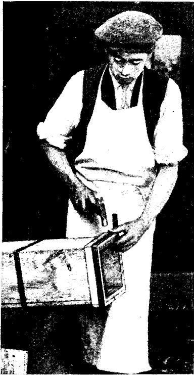
Fig. 3. Fitting the iron hoops to strengthen the joint at a section
