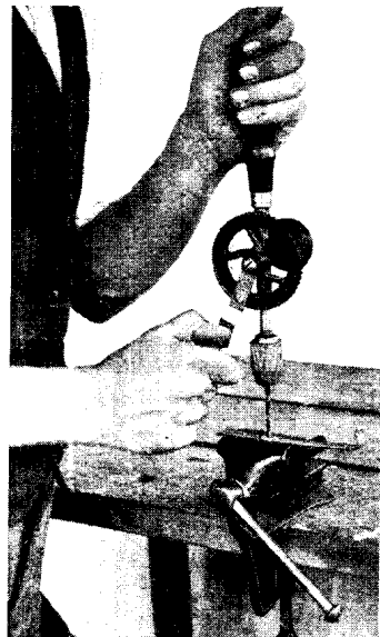
Fig. 5. Small articles made by the wireless experimenter can be drilled with a hand drill stock
