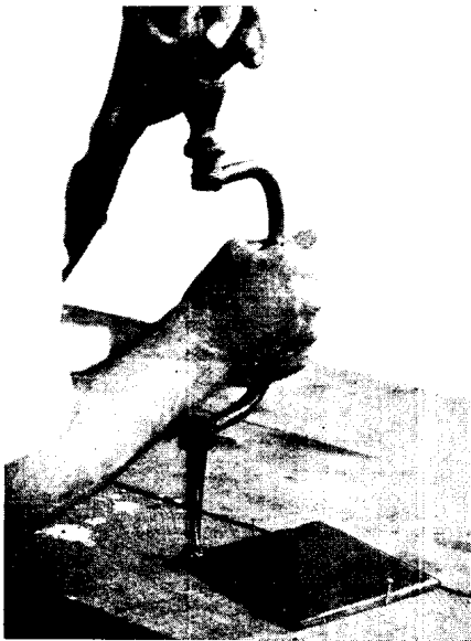
Fig. 3. How to hold the brace when countersinking a screw hole is illustrated
