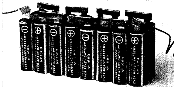
Fig. 3. Pocket lamp batteries are here seen connected in series with copper strip connexions. Note that the positive and negative terminals are joined together alternately
