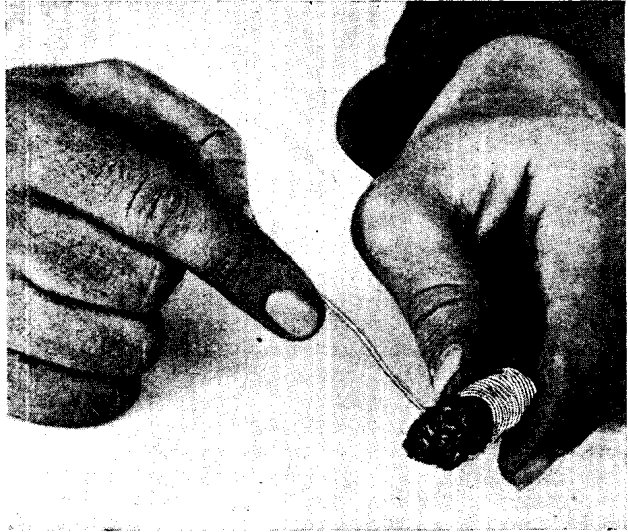
BINDING WIRE TO PREVENT FRAYING
