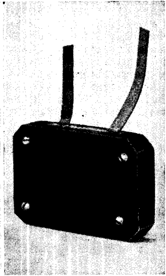
Fig. 4. Only the contact strips are allowed to protrude when the case is screwed down
