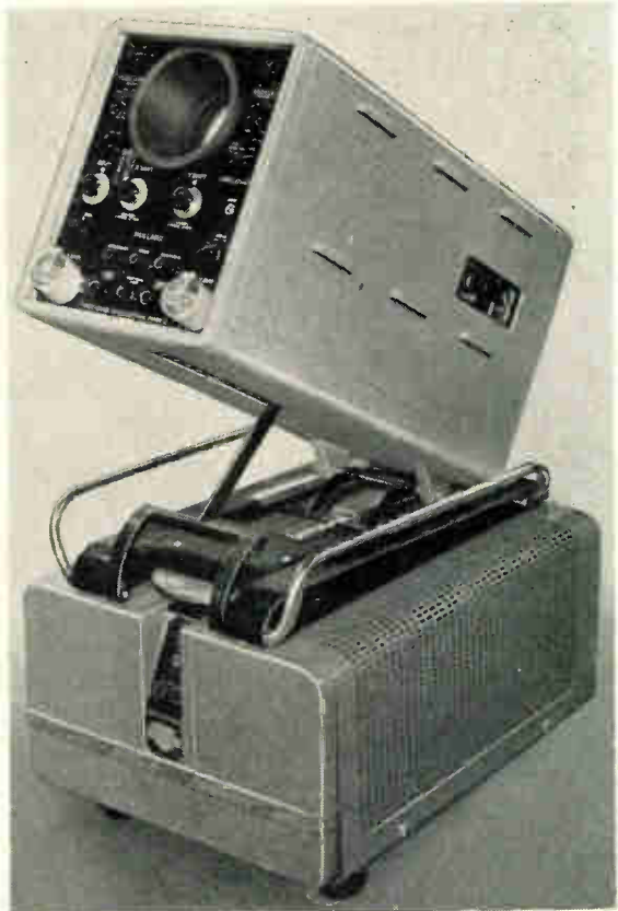
Mullard wideband oscilloscope, Mk. 11 standing on its power-supply unit.
