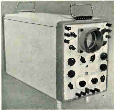
Furzehill oscilloscope intended for general-purpose use and in connection with servo systems.
