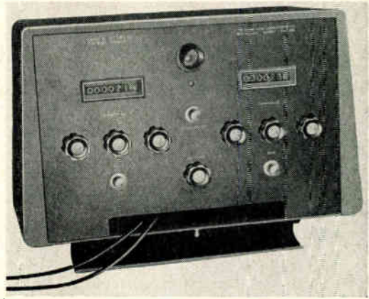
Wayne Kerr capacitance and conductance bridge with direct-reading scales.
