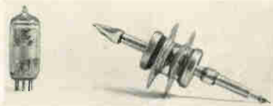
G.E.C. magnetrons; (left) 3-cm type VX3238, (right) 10-cm type VX3209.
