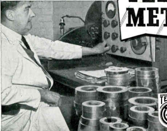
Routine Factory testing of Mumetal toroidal cores.
