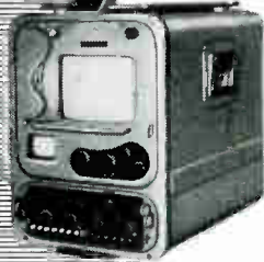
Marconi Four Channel Vision Mixer Type BD.633 with Picture and Waveform Monitor.
