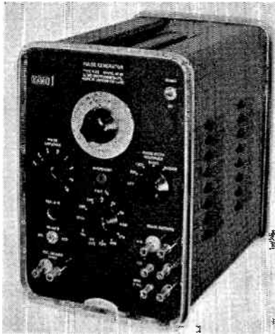
The Dawe Instruments type 412B provides twelve fixed p.r.f.s, but by connecting an external resistor or capacitor p.r.f.s. from 0 c/s to 100 kc/s can be obtained. Pulse durations are 0.3 \mu sec to 60 msec
