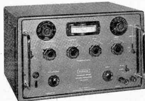
Muirhead-Wigan D-650-B 1 c/s-111,100-c/s decade oscillator. The frequency is read off four decade dials and the output voltage is monitored at all times on the panel meter
