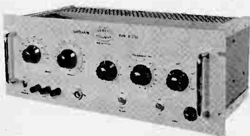
Siemens Edison R.2125 low-frequency oscillator covers the range 1 c/s-132 kc/s. The oscillator, of the Wien-bridge type, is designed primarily for a balanced output but may be operated with a single-sided output
