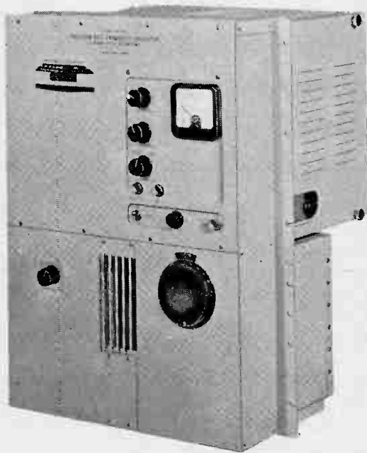
Sullivan 10A b.f.o. covers the range 0-16,000 c/s. Stability for a period of a day usually better than \pm 0.5 c/s and output level constant to within 0.1 dB
