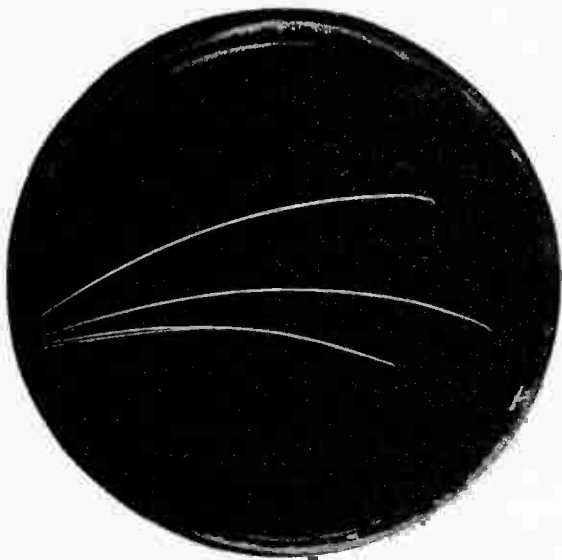
Fig. 2. Curvature of \alpha -particle tracks in a very strong magnetic field, applied perpendicular to the plane of the picture and directed upwards
