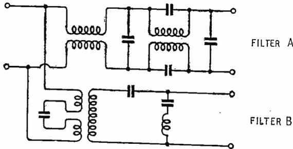
Filter A is a balanced low-pass filter with a cut-off frequency of 3 kc/s, a characteristic impedance of 600 Ω, and no physical earth connection. Filter B is a high-pass filter with a cut-off frequency of 3.5 kc/s and a characteristic impedance of 600 Ω. It has a balanced input where it is connected to the low-pass filter, but one of the coils is used as a transformer and an unbalanced output is provided.
