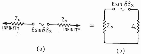
Fig. 2. Equivalent circuit in transient state of aerial having characteristic impedance  $Z_0$ .
