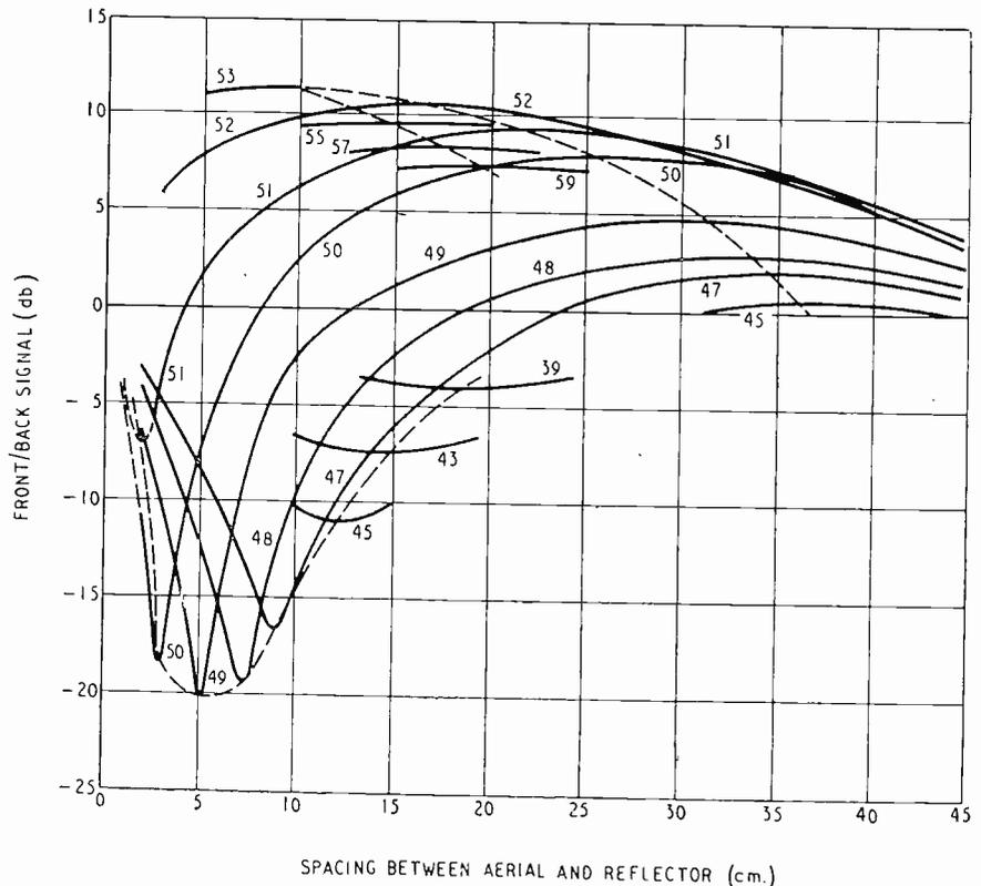
Fig. 11. *Front/back signal with various reflector lengths.  $\lambda/2$  dipole aerial.  $\lambda = 1.05$  metres. The numbers on the curves represent reflector lengths.*
