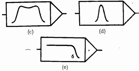
except to show how it could be included in the scheme. It will be sufficiently obvious that the combination of the rectangle with the usual triangular sign removes any possible ambiguity, as well as providing a uniform and valuable method of representing amplifiers comparable with the method for representing filters already discussed.
