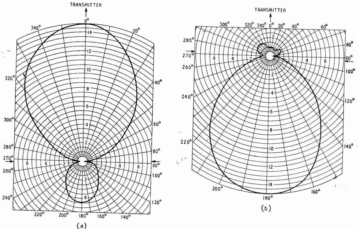
Fig. 13. Polar diagrams for a dipole with reflector (a) and director (b), at a wavelength of 105 cm. The reflector length was 53 cm spaced 18 cm from the dipole and the gain over the simple dipole was 2.9 db. The director had a length of 49 cm spaced 5 cm from the aerial and had a gain of 2.2 db over a simple dipole.
