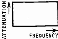
The general form of the attenuation - frequency characteristic is drawn and cut-off frequencies in kc/s are inserted in the acute angle. The characteristic impedance is written over the pass-band.
