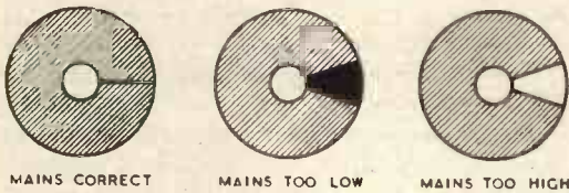
Fig. 9 (above). The illuminated target of the visual mains voltage indicator.
