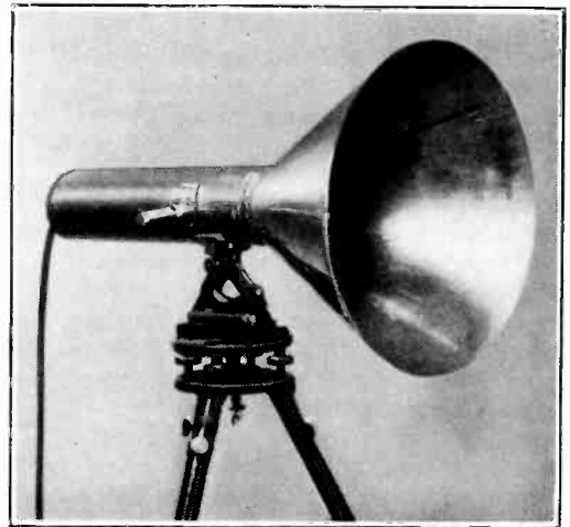
Horn and receiver for 10 cm. waves.
