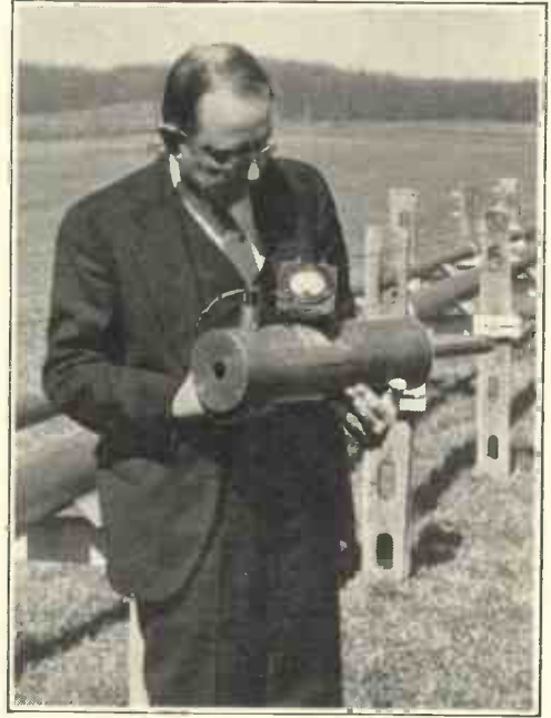
Fig. 2.—One of the resonant chambers which provide the means of tuning being examined by Dr. Southworth.
