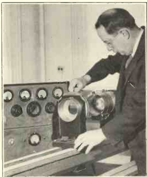
Fig. 4.—The Iris diaphragm, which provides the coupling between the transmitter and the line, can be adjusted as shown in the photograph.
