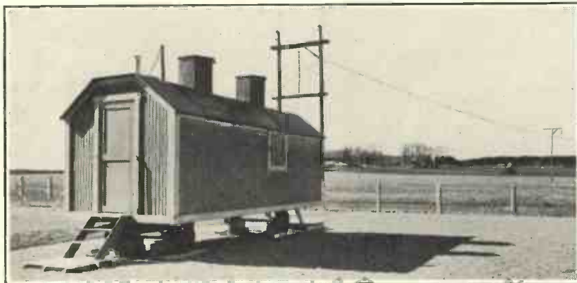
Fig. 1.—A field station for recording atmospheric on a transmission line.
