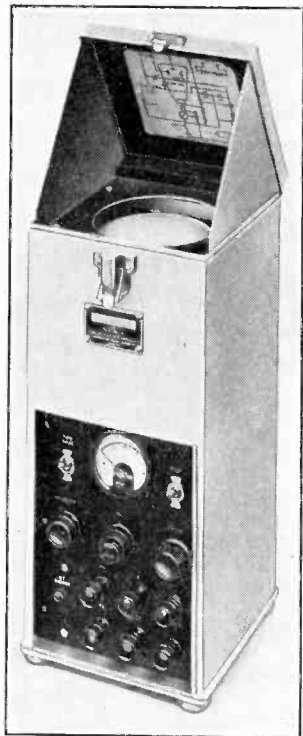
Standard Telephones cathode ray unit in which both filament current and HT voltage are derived from a 2-volt accumulator.
