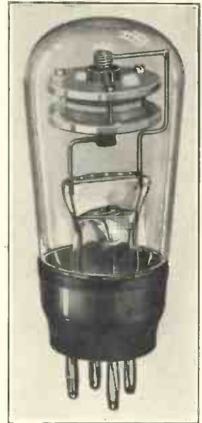
"Hivac" quartz oscillator mounted in vacuo.
