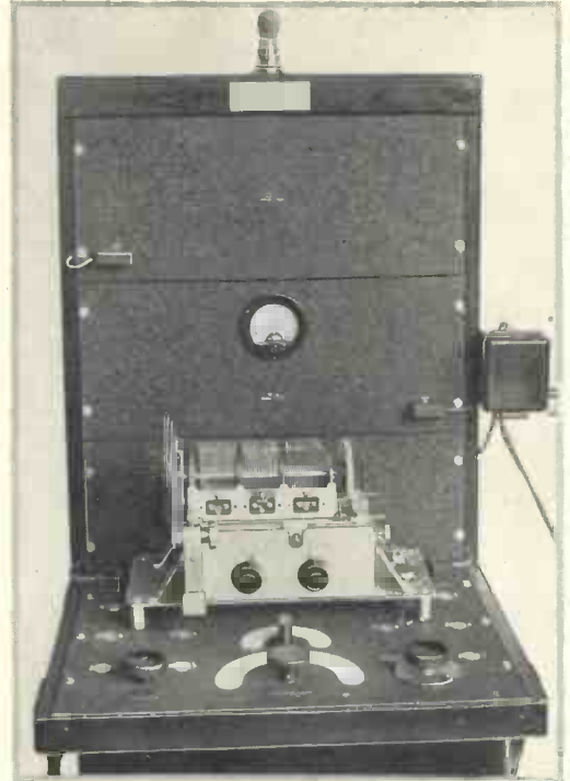
Capacity-matching bridge for works adjustment of gang condensers (E. K. Cole, Ltd.).
