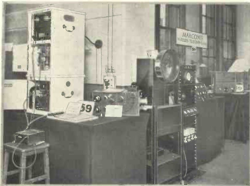
The application of high frequency currents in medical and surgical diathermy was an interesting feature of the Marconi Company's display at the recent Physical Society Exhibition. The special oscillator developed for this purpose is on the extreme left of the photograph which also shows the television photocell and reflector with its associated amplifier. The latter has a characteristic substantially flat form 10 cycles to 150 kilocycles.
