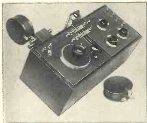
Sullivan-Griffiths universal wavemeter with interchangeable valve voltmeter and dynatron oscillator units.
