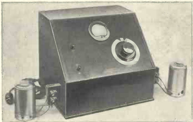
Sullivan inductance matching set for comparing screened or open coils.
