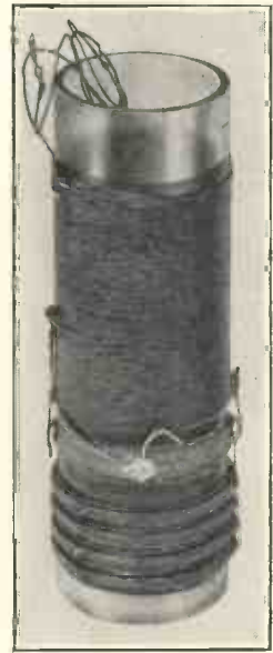
Litz-wound tuning coils on glass formers are a feature of this year's Philips' sets.
