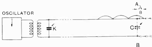
Fig. 4.—Characteristic impedance measurements.
