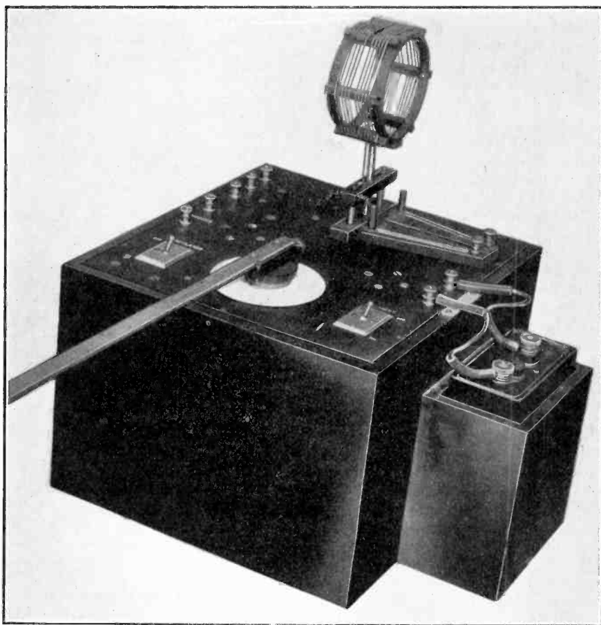
General view of the complete wavemeter
