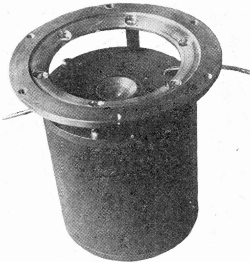
Fig. 5—Showing air gap in the core.
