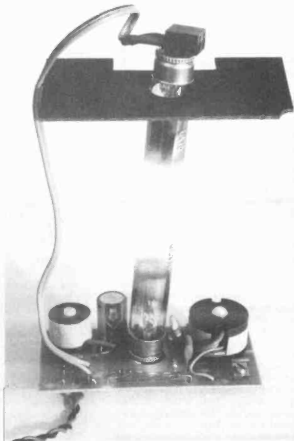
The completed circuit board, with the u.v. tube, prior to sliding it into the case side runners.
