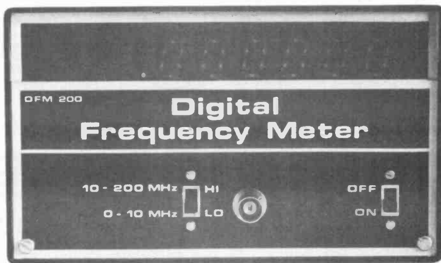
Front panel layout and legend for the 200MHz Digital Frequency Meter.
