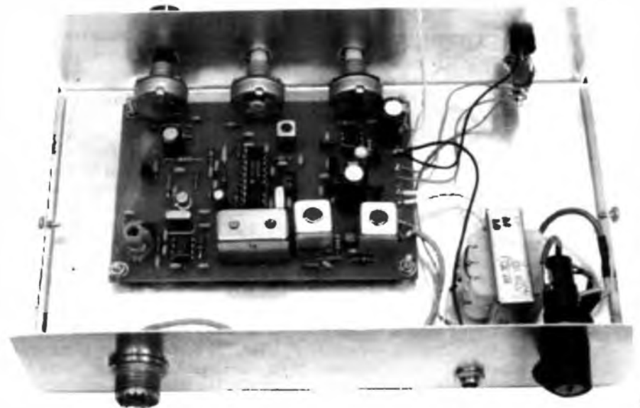
Layout of components inside the metal case. Note the loudspeaker is mounted on the underside of the case lid behind a series of "sound holes".
