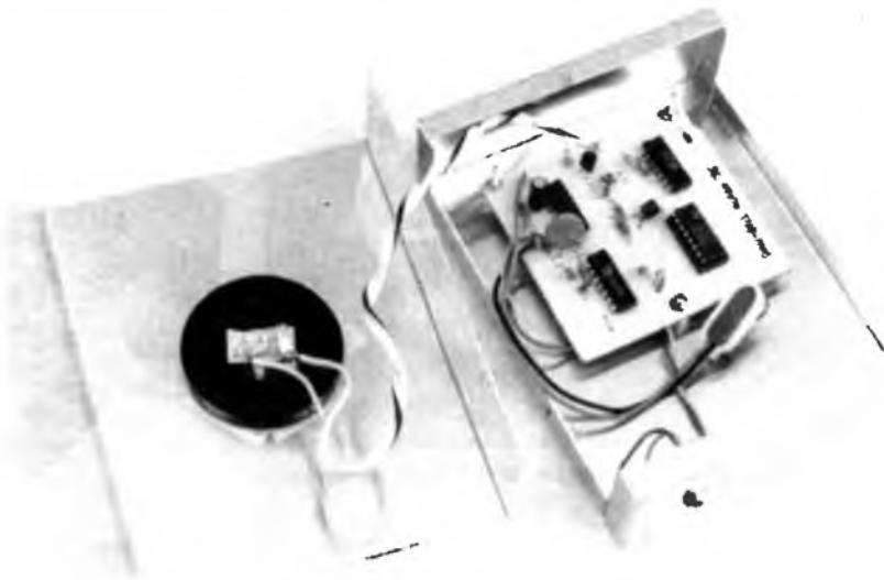
Layout of components on the two halves of the metal case.
