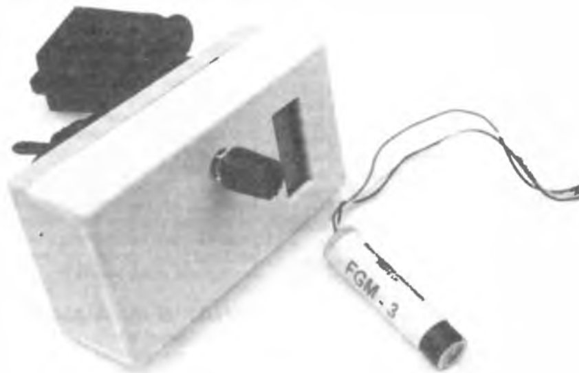
Completed Wheelie Meter with FGM-3 magnetic field sensor.
