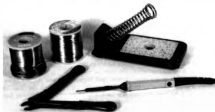
All that is needed to assemble circuit boards: two sizes of solder, small electric iron with stand and wire cutters/strippers.
