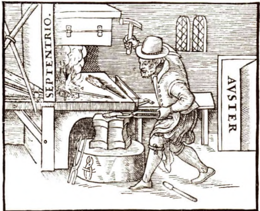
Magnetising an iron rod, as illustrated in William Gilbert's De Magnete , 1600.
