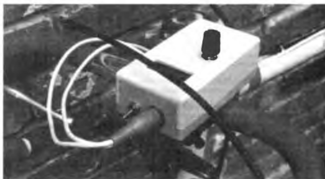
The display/control unit clamped to the bike handlebars. The two leads from the DIN plug go to the sensor and battery (located in rear saddle-bag).
