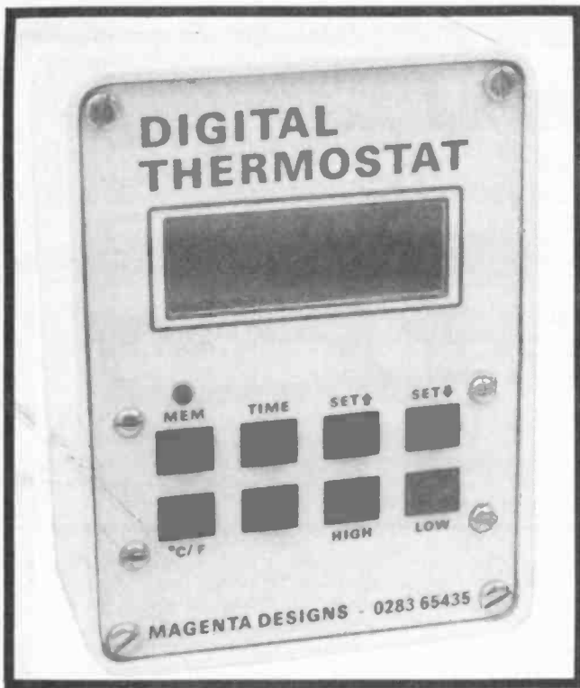
Front panel of the Digital LCD Thermostat showing the layout of the "programming" buttons and display window.
