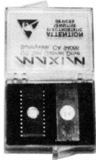
Typical anti-static plastic case and conductive foam. May be used with larger or more expensive i.c.s.
