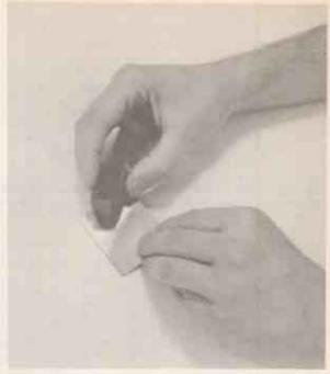
Copper-clad board, cut to size, being cleaned with an abrasive cleaning block.
