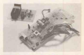
(Left) Typical single-sided printed circuit board - note the p.c.b.-mounted battery holder. (Right) A double-sided p.c.b. the copper tracks on the upper side and the through-pins can clearly be seen.
