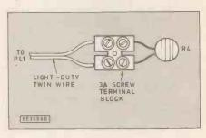
Fig. 4. Suggested method of mounting the thermistor inside a small box using a two-way terminal block.
