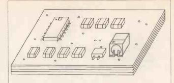
Fig. 4. A multi-layer printed circuit board, comprising of several double-sided boards bonded precisely together. Plated-through holes connect both sides of the layers as necessary.
