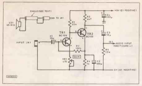
Fig.3 Additional pre-amplifer for use with the EE Telesound in order to provide "baby listening" facilities.
