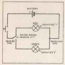
Fig. 6. Binary sending circuit.
