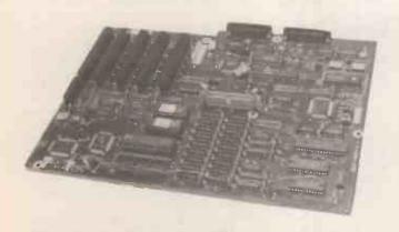
A double-sided p.c.b. combining many dual-in-line (d.i.l.) and four surface-mounted (SM) devices. This is the main board of a Victor Personal Computer.
