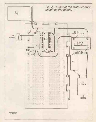
half supply voltage (4.5V) is Logic 0. This means that while the light level remains bright, the input is interpreted at Logic 0 and the output of the gate will be Logic 1 -9V – since it is a NOT gate and inverts the input.
