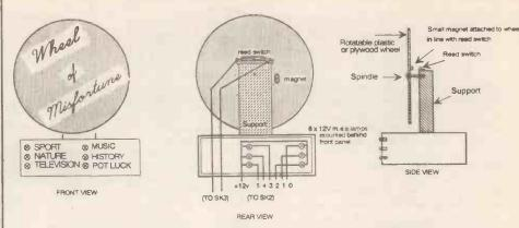
Fig. 6. Assembly and wiring to the Wheel of Misfortune display.
