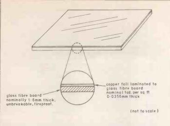
Fig. 5. Cross section of a typical copper-clad printed circuit board prior to processing.
