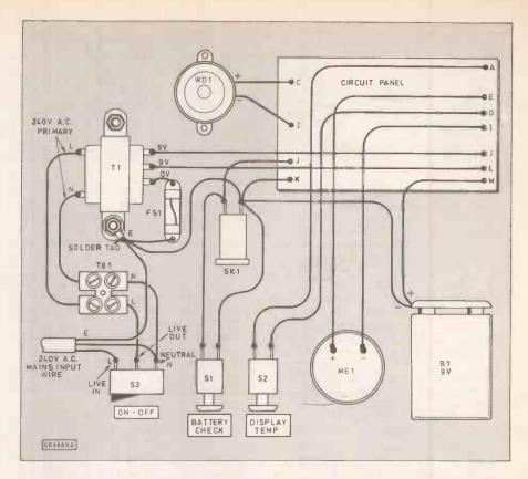
Fig. 3. Interwiring from the circuit board to the case mounted components. Mains 3A wire should be used for connecting the illuminated On/Off switch to the screw terminal block TB1. The completed unit, with cover\_removed, is shown in the photograph below. The thermistor is housed seperately in a small plastic box.
