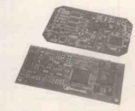
(Below) A surface-mounted p.c.b. - note the flat-pack SM integrated circuits and the tiny capacitor and resistor "chips". (Above) A commercial 4-level multi-layer p.c.b. prior to fitting with components. The darker tracks which can just be seen are actually within the board itself.
