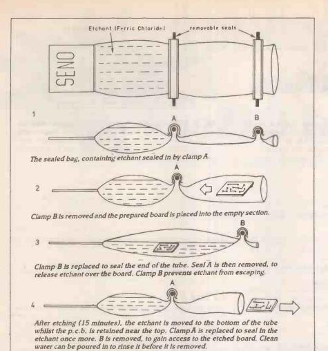
With use the Ferric Chloride solution will eventually become laden with iron, slowing down the etching time and when the etchant has finally been exhausted, a neutralising powder (supplied) is added to the solution which is eventually transformed into a solid mass for safe disposal.
