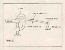
Fig. 1. Experimental "cantilever" type Load Cell set up.
