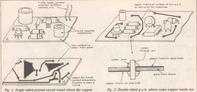
Fig. 1. Single-sided printed circuit board where the copper tracks are all on one side of the board. The components are soldered to the copper pads to form a complete circuit.
