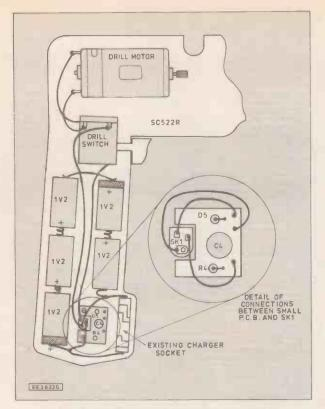
Fig. 3. Modification to the SC522R drill.
