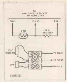
Fig. 8. L.D.R. circuit connected to a BBC Micro.
