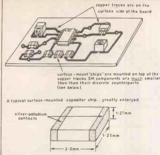
Fig. 3. Illustrating the principles of Surface Mount Technology. Very complex circuits can now be built using SM integrated circuits which occupy a very small board. The small sizes of the parts require some soldering skill
