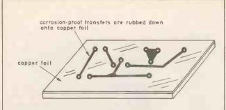
Fig. Fig. 6. Etch-resistant transfers are applied to the clean copper foll, in the desired layout of the copper track pattern. This is the "direct etch" and simplest method, of producing a p.c.b.
