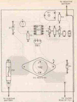
Fig. 6. Main p.c.b. construction.
