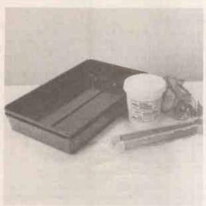
Materials for etching printed circuit boards: plastic trays, Ferric Chloride crystals, plastic tongs, goggles and disposable gloves.
