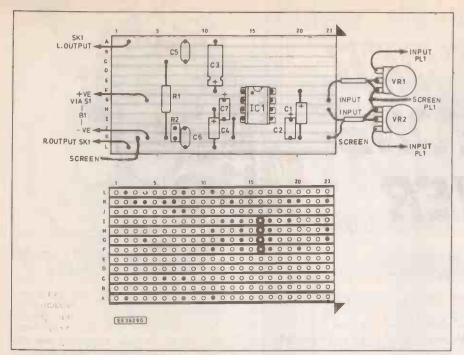
Fig. 2. Stripboard layout and wiring for the Camcorder Headphone Amplifier. Fig. 3 shows S1/SK1 wiring.
