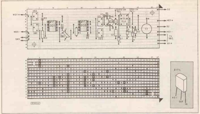
Fig. 2. Stripboard component layout and details of breaks required in the underside copper strips. The leadout details for the voltage regulator IC3 are shown on the right.
