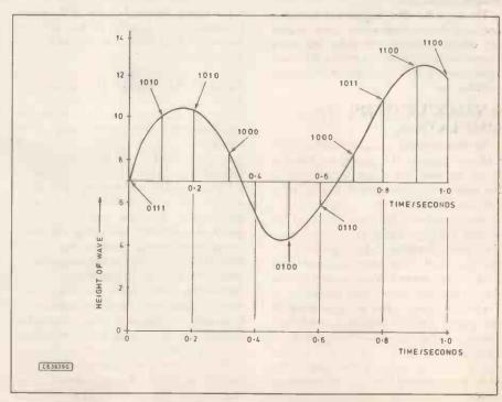
Fig. 5. Sampling the height of an analogue wave.
