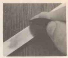
Photo 2 (above) - Using a wet/dry paper disc to abrade the metal strip.
