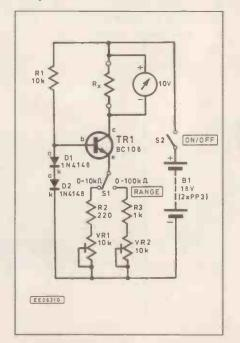
Fig. 2 Complete circuit of the linear scale ohmmeter.
