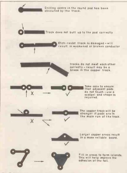
Fig. 7. Pitfalls when applying etch resist transfers to a p.c.b. The same problems can arise when preparing artwork for use with the ultra-violet method, described fully next month.
