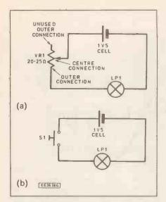
Fig. 4. Analogue (a) and digital (b) circuits.
