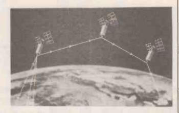
When placing a call on the Motorola Iridium System, the signal is transmitted from the caller's portable cellular phone directly to the nearest overhead satellite, which in turn sends the signal to an earth "gateway" station that verifies the caller as an authorised user. The call is then routed through the constellation of satellites to its destination anywhere on earth.
