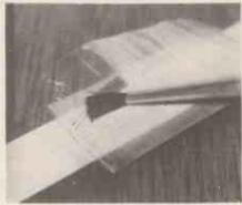
Photo 4 - Use a small art brush to apply a thin layer of activator liquid.
