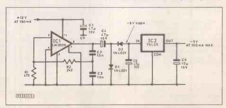
Fig. 5 Complete - 5V 100mA power supply based on an LM380.
