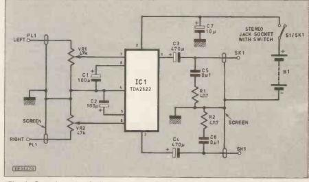
Fig. 1. Complete circuit diagram of the Camcorder Headphone Amplifier. The text refers to S1/SK1.
