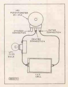
Fig. 3. Practical layout for the analogue circuit.
