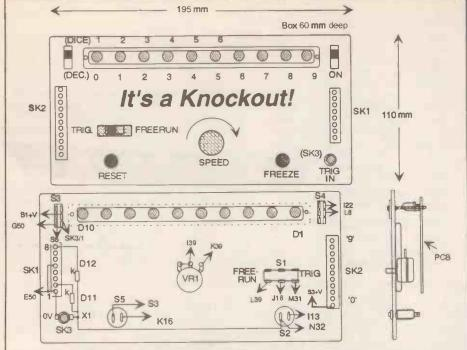
Fig. 3. Front panel layout and wiring from panel mounted components to circuit board. Letters and numbers are board grid references.
