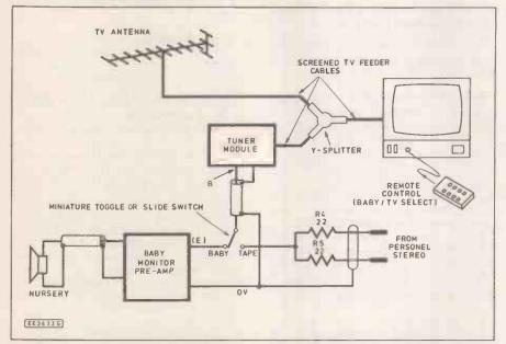
Fig.4 Method of connecting the EE Telesound to provide switching between TV programmes and baby listening.
