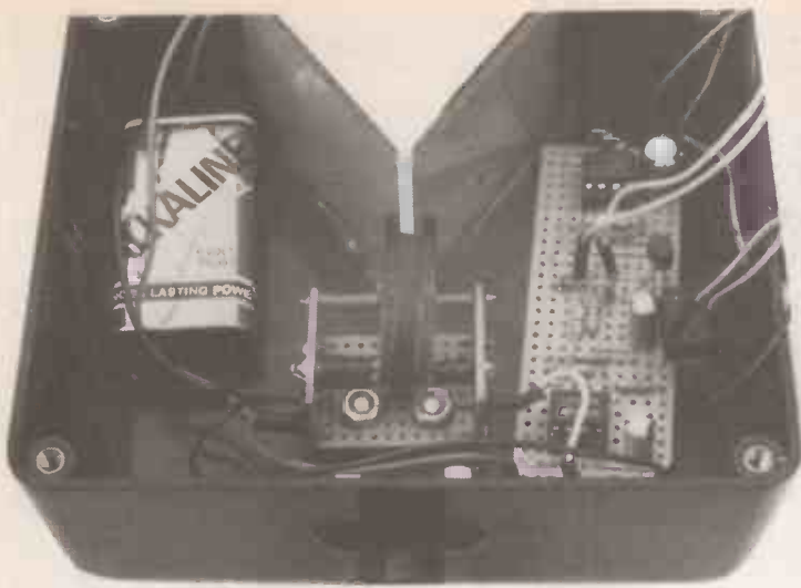
Mounting the sensor chassis so the wheel aligns with the "rod line" V-slot.
