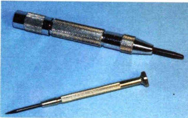
An automatic centre punch (top) is ideal for use with aluminium but should not be used with plastic. Instead use a sharp bradawl or stiletto (bottom) with no more than moderate pressure.
