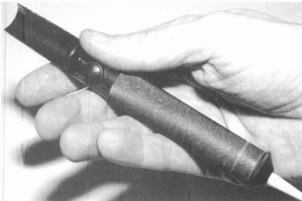
A typical solder pump; the nozzle is seen at the right and the release button is just below the thumb.
