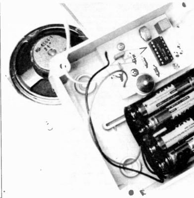
Layout of components inside the waterproof case. The loudspeaker is glued to the inside of the lid.
