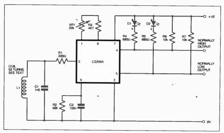
Fig. 10.4. Example circuit diagram for using the CS209A.
