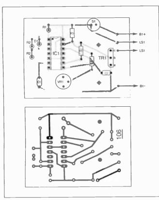
Fig. 3. Printed circuit board component layout and full size underside copper foil master pattern.
