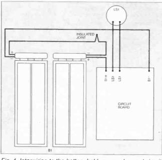
Fig. 4. Interwiring to the battery holders, speaker and circuit board.
