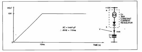
Fig. 3. Charging a capacitor through a constant current source.
