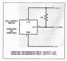
Fig. 10.2. Biasing the output.
