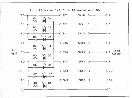
Fig. 1. The circuit diagram for a simple RS232CC breakout box.
