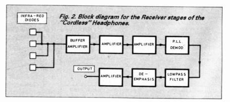
The total average l.e.d. current is about 250mA, and the current consumption for the entire circuit is approximately 260mA. This is too high to permit battery operation, and the unit must therefore be powered from a mains power supply unit. This must provide a well smoothed and regulated 12V output. The circuit diagram for a suggested power supply is shown in Fig. 4.
