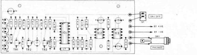
Fig. 8. (above) Circuit board component layout and wiring, and (right) actual size copper foil master for the Headphone Receiver.
