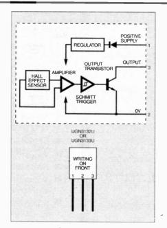
Fig. 10.1. Block diagram and pinout details for Hall effect sensors type UGN3132U and UGN3133U.
