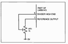
Fig. 10.11. Adjusting the bargraph response range.
