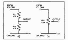
Fig. 10.10. Changing the output level from IC1 in Fig. 10.9.
