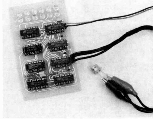
Completed Component Analyser p.c.b. with a transistor in the "jaws" of the crocclips ready for testing.
