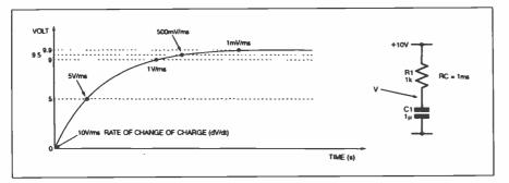
Fig. 2. Exponential charge curve of a basic R-C network.
