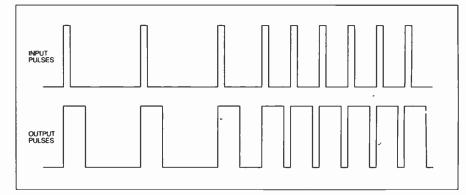
Fig. 10.6. Relationship of monostable input and output pulses.
