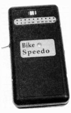
brand new bike, but the slightest imperfection in the geometry of the wheel could cause sensing problems. The chosen method of sensing the rotation was to use the proximity sensor i.c. type CS209A.
