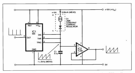
Fig. 4. Ramp generator using constant current regulator diode in a 555 oscillator.
