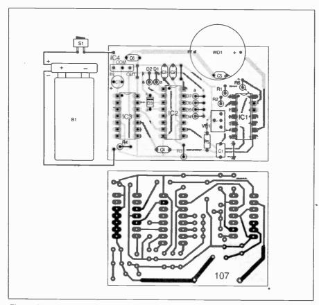
Fig. 3. Mobile Miser printed circuit board component layout, full size copper foil master pattern and switch and battery wiring.
