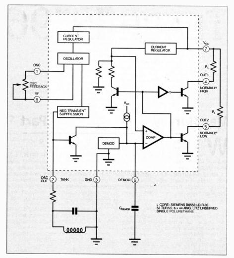
Fig. 10.3. Functional block diagram for the CS209A proximity detector.
