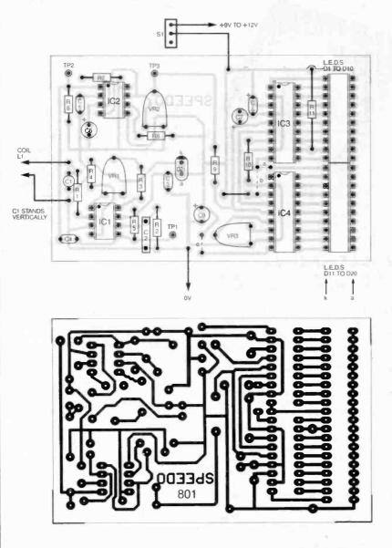
Fig. 3. Printed circuit board component layout and full-size underside copper foil master track pattern.
