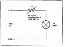
Fig. 1. Simple bulb protector.
