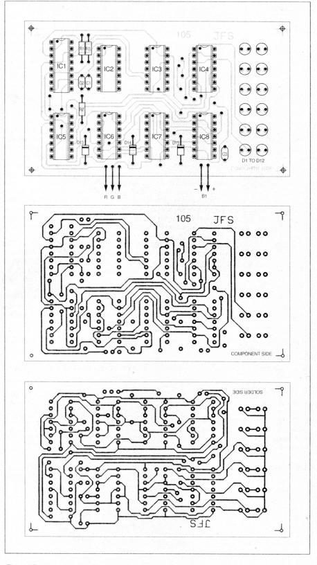
Fig. 3. Printed circuit board component layout and full size top and bottom copper master patterns. This board is a "plated-through-hole" type, see text.
