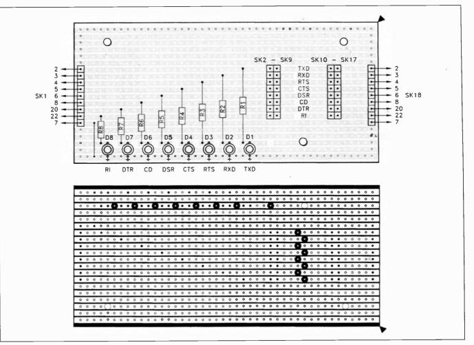
Fig. 2. Suggested stripboard construction of the circuit in Fig. 1.
