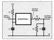
Fig. 10.5. Basic frequency to voltage conversion using a monostable.
