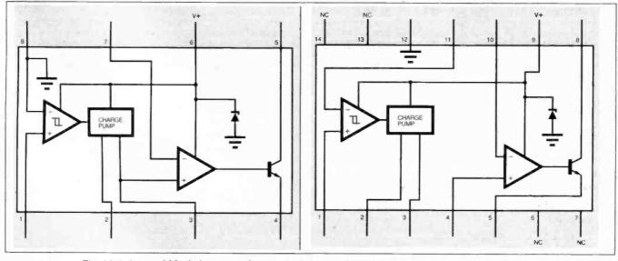
Fig. 10.8. Internal block diagrams of the LM2917N-8 (left) and LM2917N (right) tachometer i.c.s.
