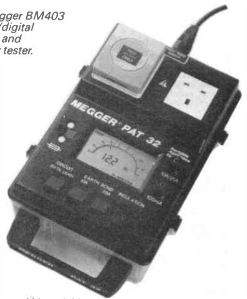
(Above) Megger PAT32 Portable Appliance Tester from AVO.
