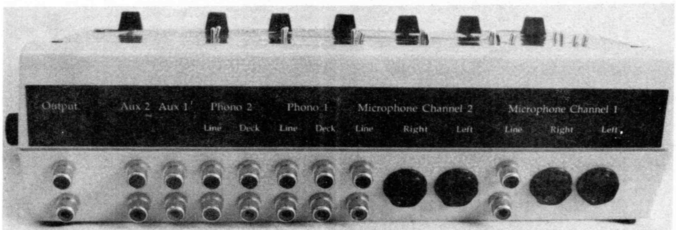
Rear view of the mixer console showing the layout of the input and output sockets.
