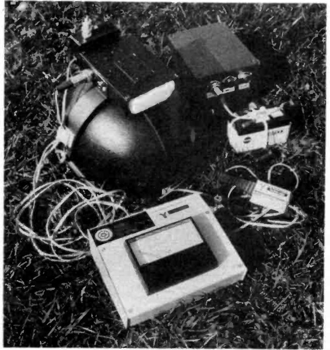
Horse speedometer electronics. The microwave "gun" mounted on the riders helmet with wrist readout, belt mounted electronics and battery, and the remote speed readout incorporating a radio data link.
