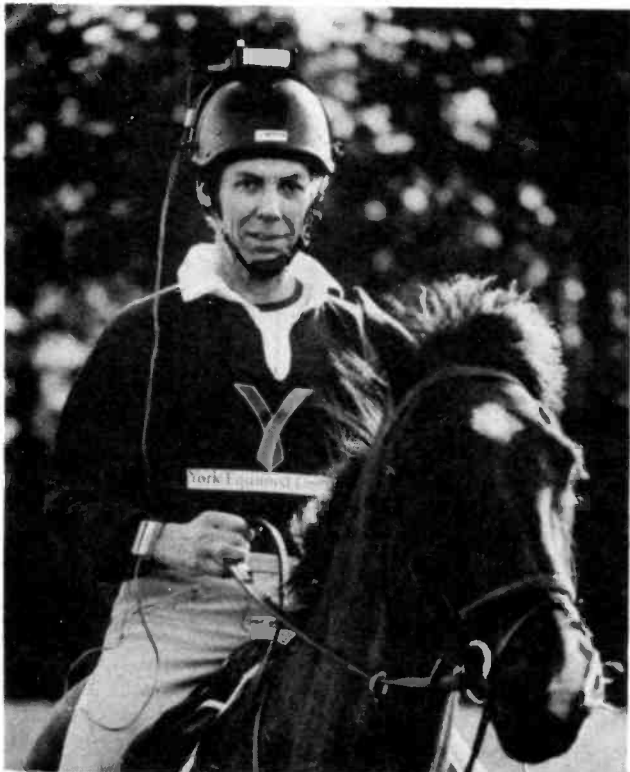
Horse speedometer electronics. The microwave "gun" mounted on the riders helmet with wrist readout, belt mounted electronics and battery, and the remote speed readout incorporating a radio data link.
