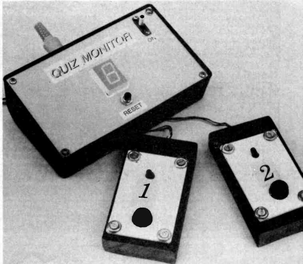
Fig. 2. Circuit arrangement for four contestant key-pads. The key-pads are wired to two DIN plugs in pairs. (below) The completed Quiz Monitor showing two prototype key-pads.
