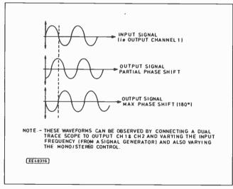
Fig. 1. Sine wave showing phase shift.
