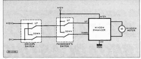
Fig. 5. Suggested possible wiring arrangement to achieve passenger/driver control of the passenger window.
