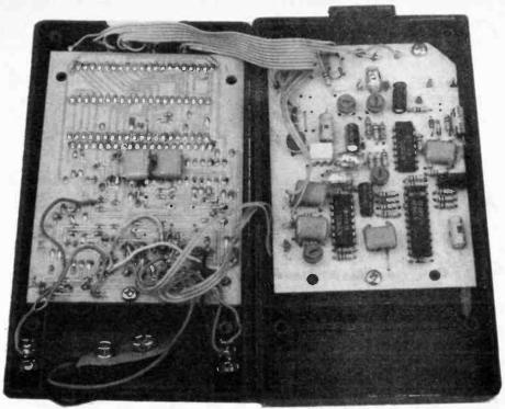
The completed Biomet opened out to show the Display and Sensor boards mounted in the hand-held case. The sensor board is the one on the right.
