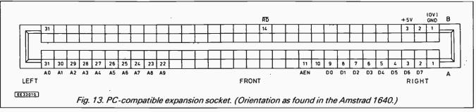
PC-compatible expansion slot shown in Fig.13, check the correct orientation for the ADC board. Insert the board carefully into the expansion slot, ensuring that the edge connector tracks line up with the slot terminals. It may be necessary to slightly file down the sides of the p.c.b. in order to achieve satisfactory alignment.
