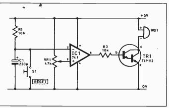
Fig. 5.5. Time delay circuit using an op-amp.
