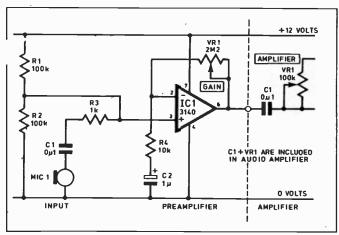
Fig. 5.10. A complete microphone amplifier system using the Mini Lab Audio Amplifier.
