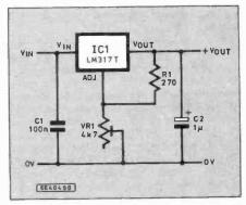
Fig. 1. Circuit diagram for the lowvoltage Add-On Board for the Personal Stereo Amp. (Nov. '92).
