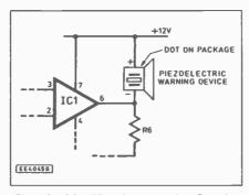
Fig. 3. Modification to the Car Ice Alarm (Jan '93) circuit to provide audible output.
