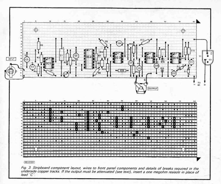
The board has 60 holes by 19 copper strips. A board of this size must be cut from a larger piece using a hacksaw. Cut along rows of holes rather than trying to cut between rows (which is virtually im-
