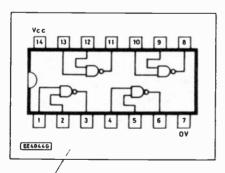
Fig. 2. Package outline and pin connection details for the 74LS00.
