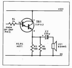
Fig. 5.7b. Loudspeaker driver circuit suitable for the oscillator of Fig. 5.7a.
