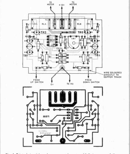
Fig. 4. Printed circuit board component layout and full size copper foil master pattern. Note the "dashed" lead-off wires are soldered directly to the underside copper pads (see text).
