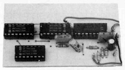
Early prototype topside component layout for the ADC Interface board. The final board is a double-sided p.c.b., see Fig. 12.
