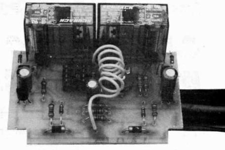
The completed printed circuit board component layout. Resistor R9 is made up from a pice of 0.6mm dia. insulated copper wire (approx 20cm), coiled up for neatness, and can be clearly seen above.
