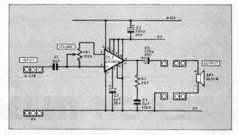
Fig. 1. Circuit diagram of the Mini Lab Audio Amplifier. The loudspeaker SP1 was fitted to the Mini Lab p.c.b. last month.
