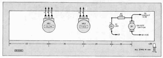
Fig. 6. Control and I.e.d. wiring diagram
