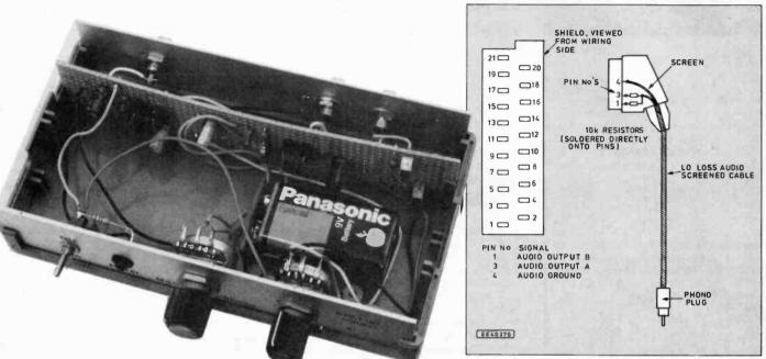
Fig. 7. Wiring of the SCART socket using two 10k resistors to combine the two signals.
