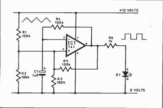
Fig. 5.7a. L.E.D. flasher/oscillator.
