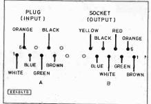
PIN FUNCTION CABLE OUT 1 = XB (RIGHT) BROUN OUT 2 = XA (LEFT) GREEN OUT 3 = YA (UP) **WHITE** OUT 4 = YB (DOWN) **BLUE** OUT 5 = NC OUT 6 = LEFT BUTTON ORANGÉ OUT 7 = +5v RED OUT 8 = GROUND BLACK OUT 9 = RIGHT BUTTON YELLOW
