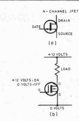
Fig. 5.14. The field-effect transistor. (a) A Junction FET. (b) A MOSFET in a simple switching circuit.
