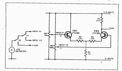
Fig. 5.1. A transistor differential amplifier.
