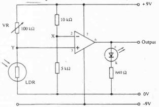
The op-amp is powered by a  $\pm$  9V supply.
