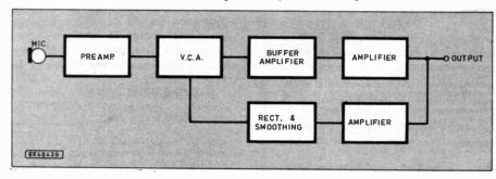
Fig. 1. Block diagram for the Microphone Compressor.
