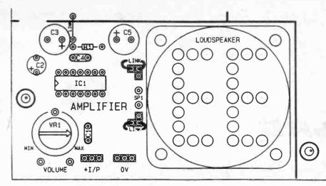
Fig. 2. Mini Lab layout for the Audio Amplifier. Two solder pins are needed at the location marked "SPI" pointing downwards, these are then connected, using insulated wire, to the loudspeaker terminals.
