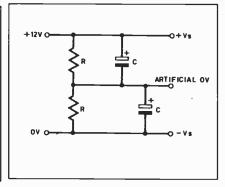
Fig. 5.9. One way of creating "artificial" split rails from a single supply.
