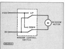
Fig. 1 (left). The conventional set-up for the driver's electric window control switch.
