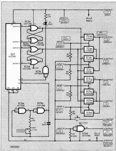
Fig. 1. Full circuit diagram for the Simplifly Atari STFM Interface. Note that the Joystick input common connection, usually connected to "ground" (0V), is taken up to the "positive" rail (+5V) – see text.
