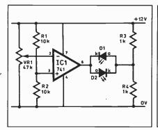
Fig. 5.8a. Sink and source capability of an op-amp.
