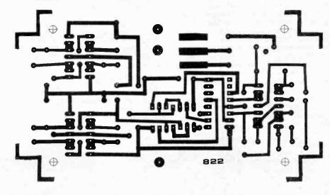
Fig. 2. Printed circuit board component layout and full size copper foil master pattern. The completed prototype board is shown below. Make sure you insert the two line wires under IC4 and IC5 before mounting the i.c. sockets, see above.
