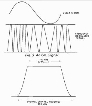
Fig. 4. Spectrum of an f.m. signal.
