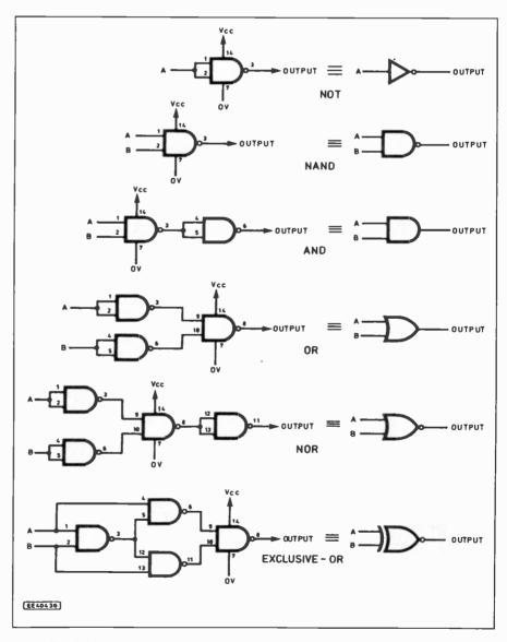
Fig. 1. Various logic functions produced by a single 74LS00 NAND gate
