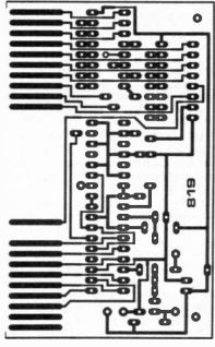
Fig. 12. The ADC Interface printed circuit board. The numbered leads from the board are soldered in the stereo jack plug JK2, see Fig. 8 and Fig. 11 (last month).
