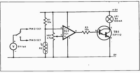
Fig. 5.4a. A light-sensitive comparator circuit.
