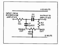
Fig. 5.11. A simple treble and bass-cut tone control circuit.
