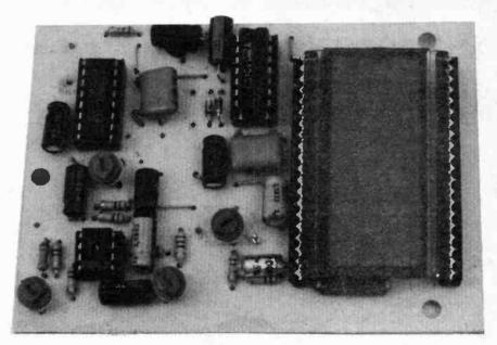
The completed Display board. Note the radial electrolytics are laid flat to save space and the display driver i.c. is mounted under the LCD.
