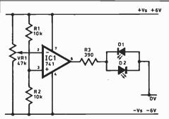
Fig. 5.8b. Use of an op-amp with dual supply rails.
