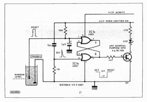
Fig. 1. Simple Washer Fluid Alarm circuit.
