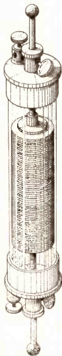
Fig. 3. Zamboni Dry Pile, 1812; invented by Abbe G. Zamboni (c1800). One of the first attempts to produce a dry cell.
