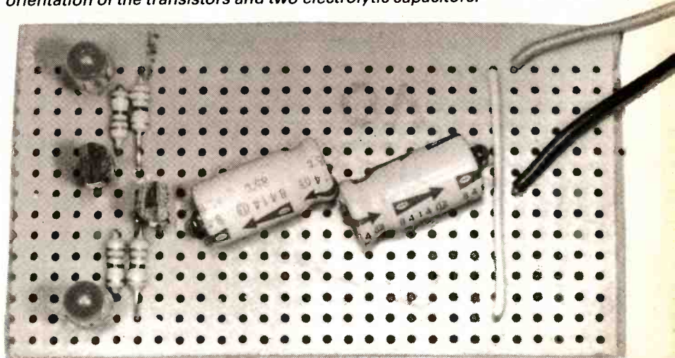
The completed circuit board showing the layout of components. Note the orientation of the transistors and two electrolytic capacitors.
