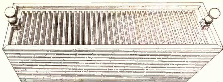
Fig. 2. Cruikshank Battery, 1800; invented by William Cruikshank (1745-1829). Davy and Faraday used batteries of this type for their major discoveries.
