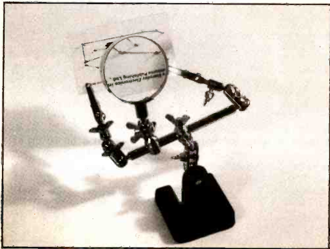
Checking a solder joint with a magnifier attached to a "helping hand" jig.
