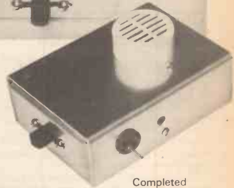
Completed alarm with thermistor protruding through rubber grommet in side of the case
