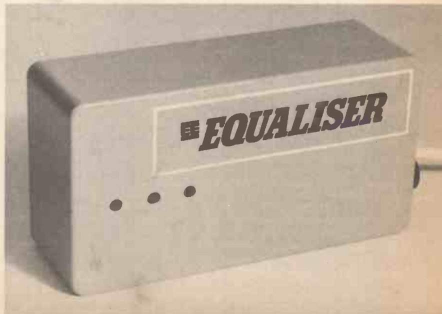
The completed unit showing the tips of the "ion" emitter pins.
