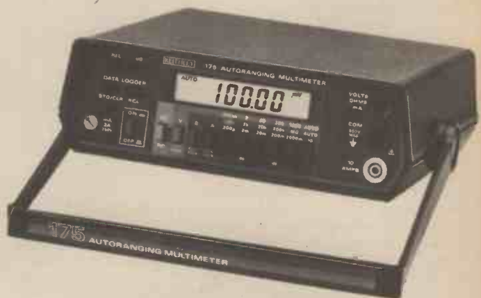
Model: Keithley 175. Ranges: 200mV–1kV d.c., 200mV–750V a.c., 200 \mu A–10A a.c./d.c., 200 \Omega –20M \Omega . (27 ranges). Impedance: 10M \Omega . Special Features: Autoranging, \mu P operated with memory (100 readings). IEEE bus. Price: £449 + VAT. Supplier: Keithley Instruments Ltd., 1 Boulton Rd., Reading, Berkshire, RG2 0NL. (0734 861287).
