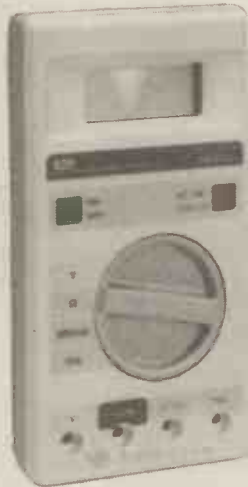
Model: Beckman T90. Ranges: 200mV–1kV d.c., 200mV–600V a.c., 200 \mu A–2A d.c., 200 \Omega –20M \Omega . (18 ranges). Impedance: 10M \Omega . Special Features: Diode test. Price: £59 + VAT. Supplier: Beckman Instruments Ltd., Mylen House, 11 Wagon Lane, Sheldon, Birmingham, B26 3DV. (021 742 7761).
