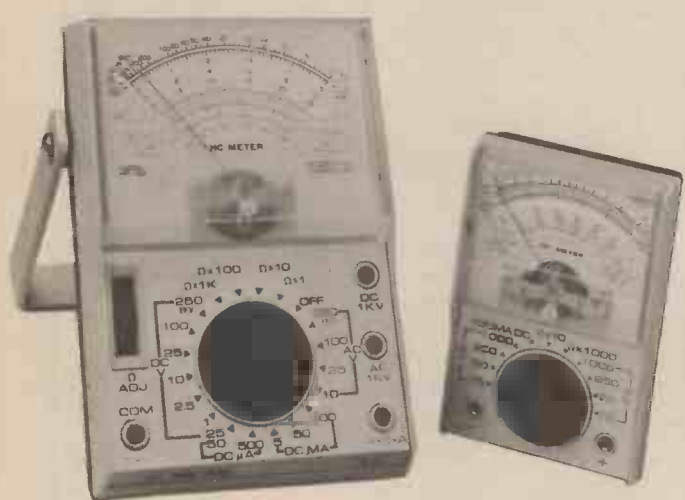
Model: Hung Chang HM101. Ranges: 10V–1kV a.c./d.c., 100mA d.c., 1M \Omega . (12 ranges). Model: Hung Chang HM102. Ranges: 250mV–1kV d.c., 10V–1kV a.c., 50 \mu A–500A, 6M \Omega . (14 ranges). Impedance: Not known. Price: £14 + VAT. Supplier: Cirkit Holdings PLC, Park Lane, Broxbourne, Herts. (0992 444111).
