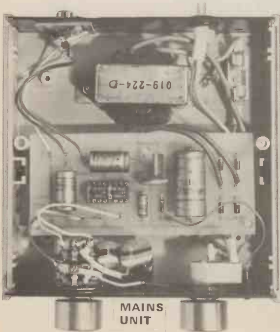
Fig. 4. Wiring and layout diagram. Note: C1 and C2 should go to the left-hand tags of VR1 and, instead, the wipers to the p.c.b.
